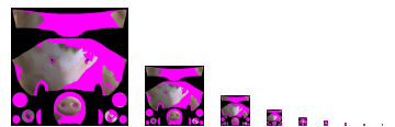
Figure 1: A sample pyramid of Primitex textures for a single frame, with invalid pixels (areas hidden from camera) rendered pink.
